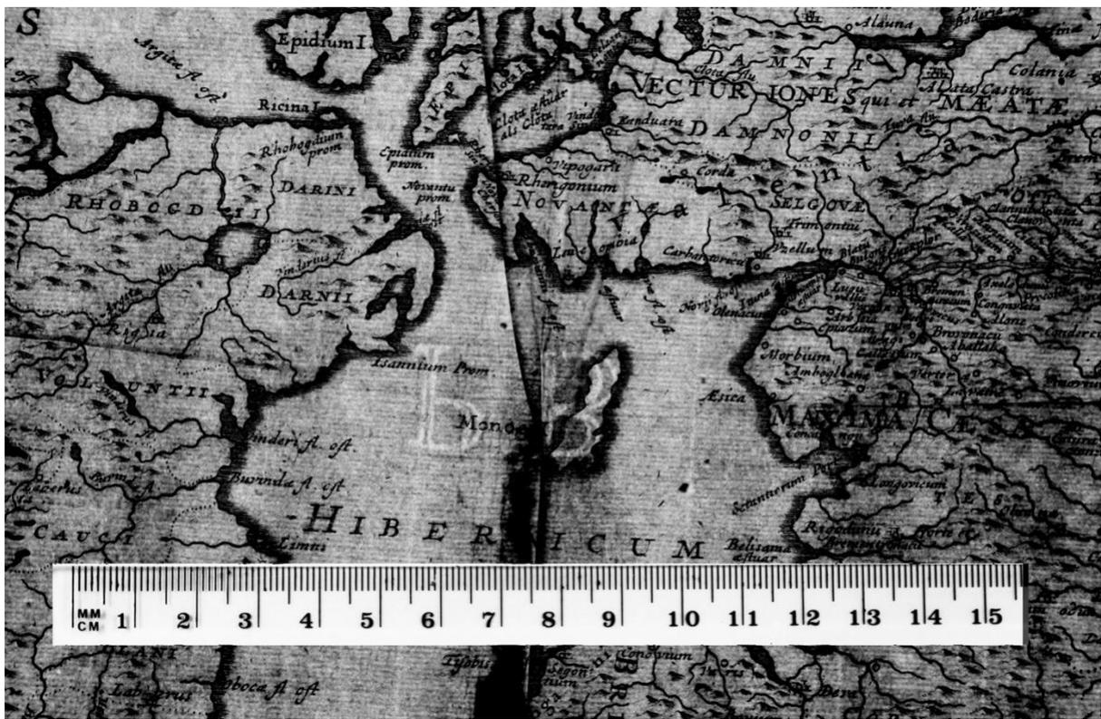
The chain lines, the laid lines and items such as specks and flecks in the paper are clearly visible. The distribution is unique to that item.
